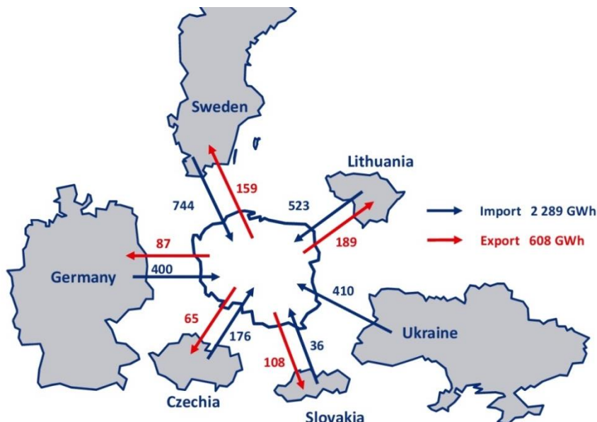
Diagram: Geographical structure of commercial exchange in the first quarter of 2019 (in GWh).
