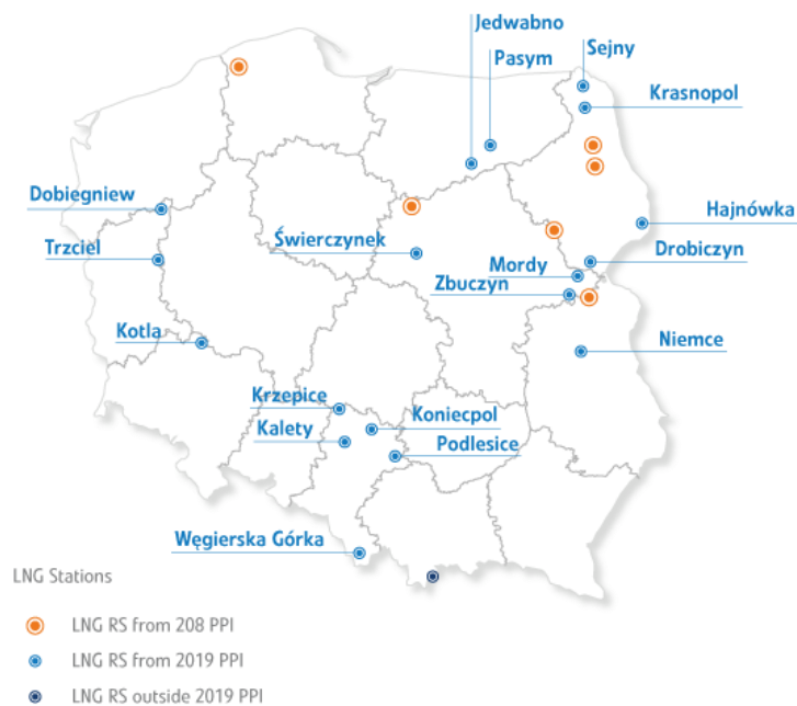
Figure 8 LNG regasification stations in Poland
